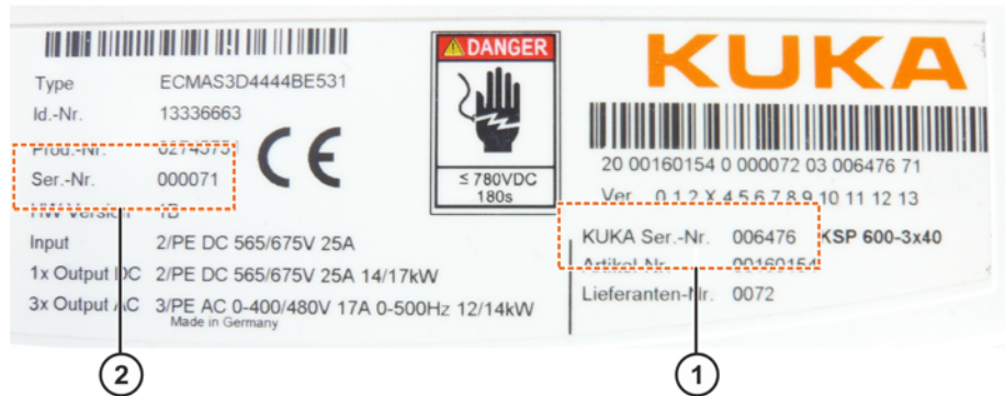
Fig. 10-4: Example: Labels on the Lenze KSP/KPP
